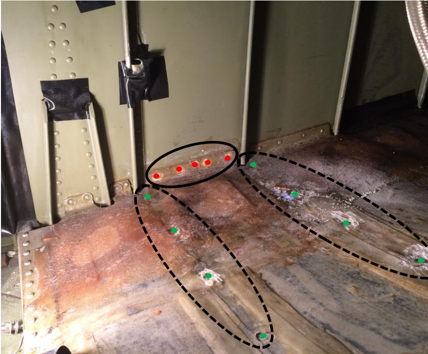
Figure 4.1.5 Rivet Removal for Fuel Tank Liner
