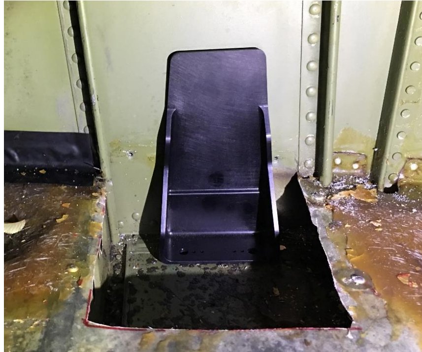
Figure 4.1.9 Lower Keel Beam – T Cap Rivets Removed
