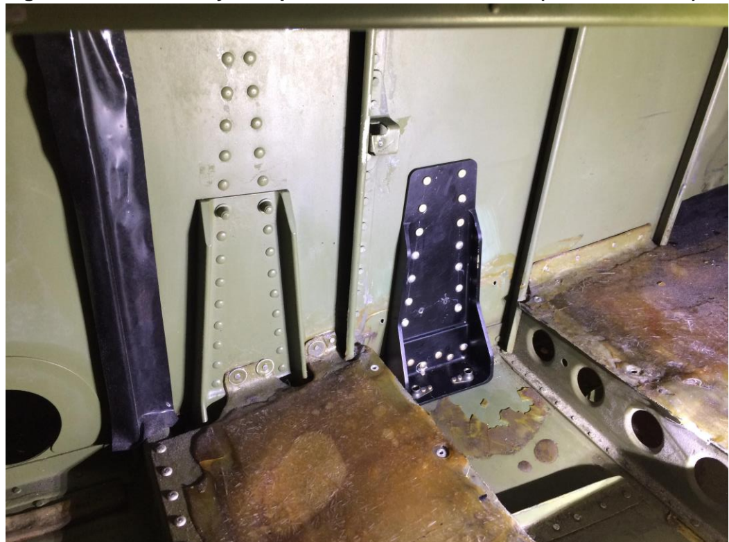
Figure 4.1.1 Secondary Hardpoint Installation Location (left side shown)
