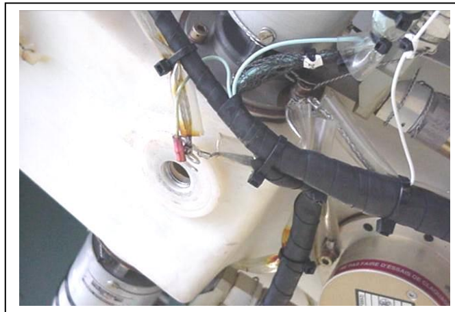
Figure 2.4.2 Fuel Drain Disassembly Complete
