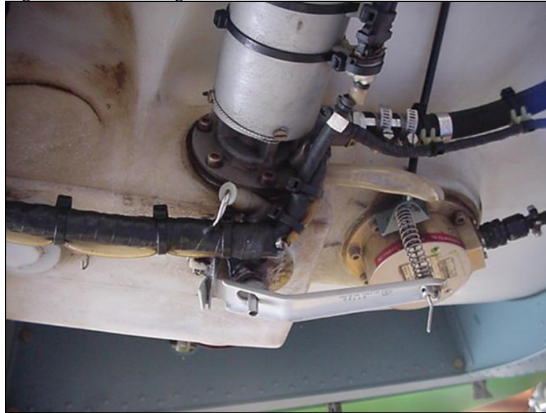
Figure 2.4.1 Removing Control Cable
