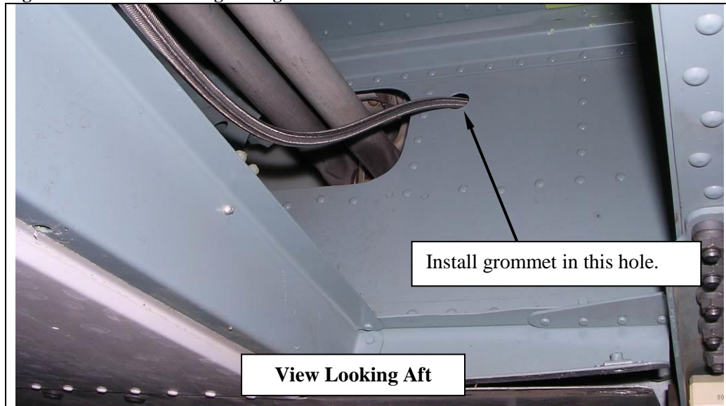
Figure 2.2.10 Hose Routing through Rear Cabin Bulkhead
