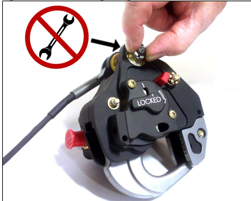
Figure 5.5 Pin Load Cell Tightening
