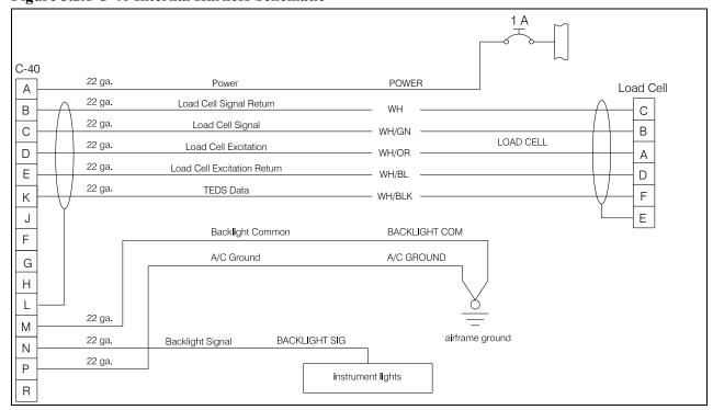
Figure 5.2.1 C-40 Internal Harness Schematic
