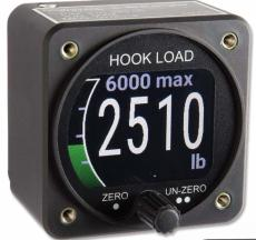
The analog bar on the left of the screen gives the pilot a way to quickly view the total weight on the hook.
