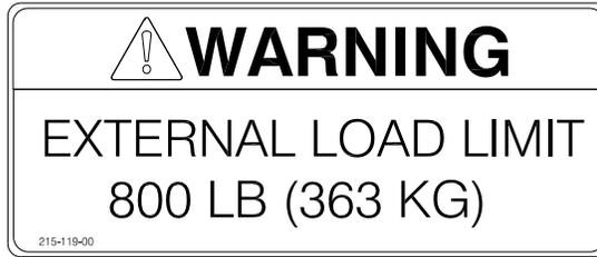
Mounted on the belly of the aircraft adjacent to the cargo hook attachment point in clear view of the ground support personnel.
