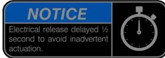
Adhered on the solenoid housing of optional cargo hook P/N 528-029-02 which is equipped with Surefire Release.
