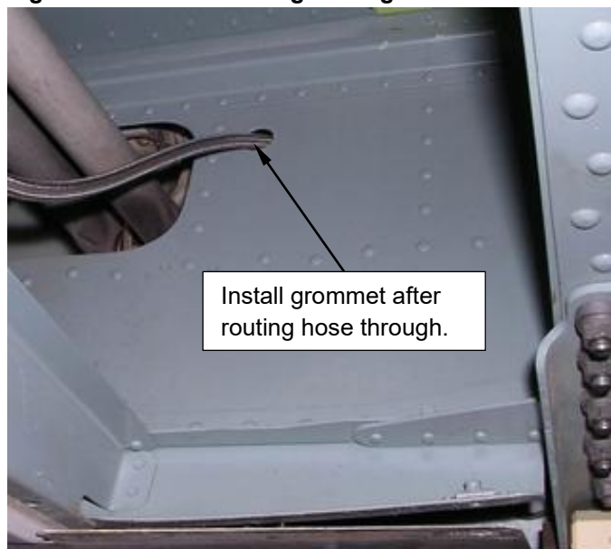
Figure 4.4.7 Hose Routing Through Aft Bulkhead
