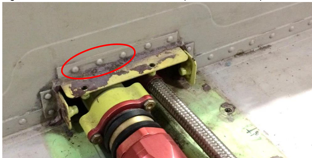
Figure 3.1.2 Brackets and Rivets to Remove (Forward Bulkhead)
