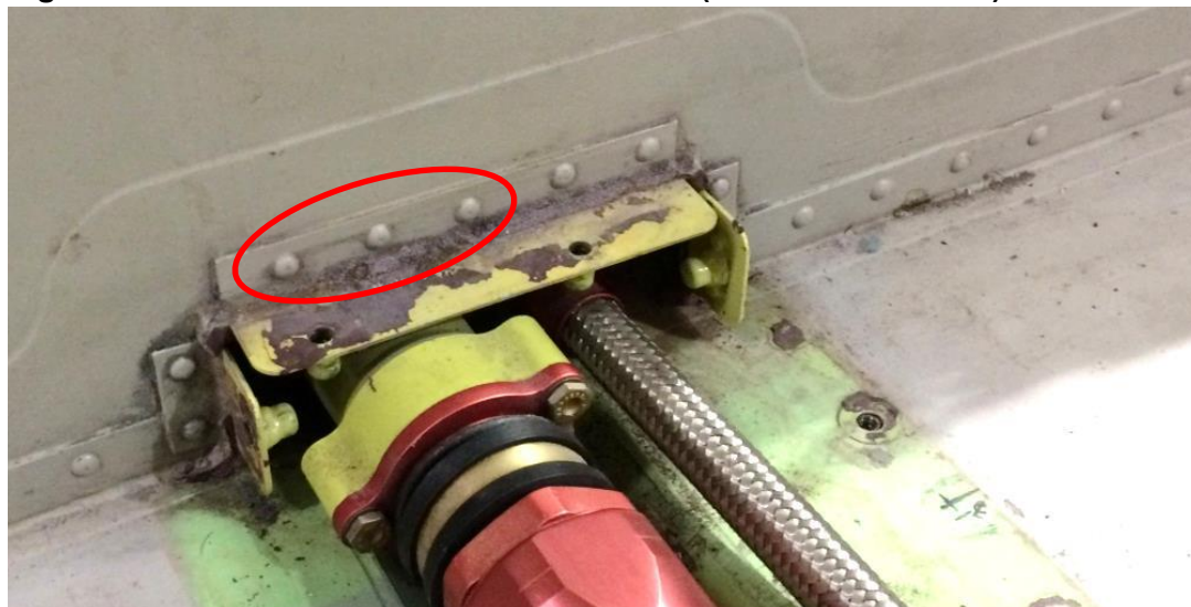
Figure 3.1.2 Brackets and Rivets to Remove (Forward Bulkhead)
