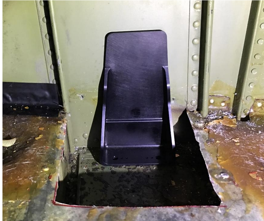
Figure 4.1.9 Lower Keel Beam – T Cap Rivets Removed
