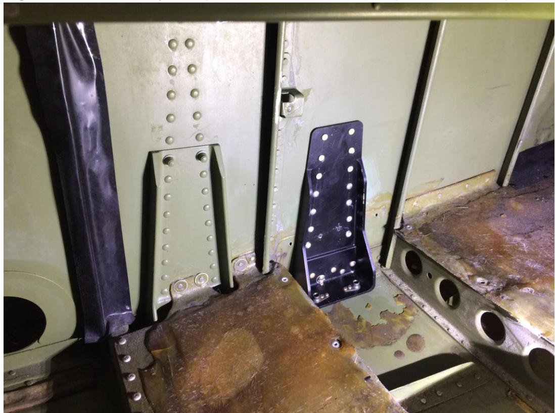
Figure 4.1.1 Secondary Hardpoint Installation Location (left side shown)
