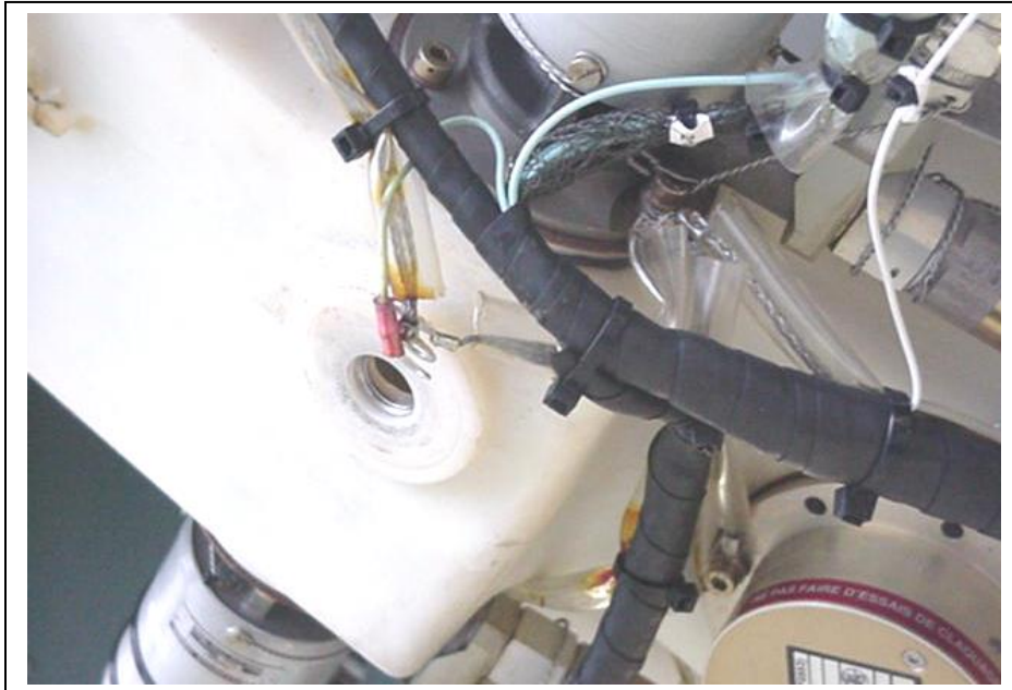
Figure 2.5.2 Fuel Drain Disassembly Complete
