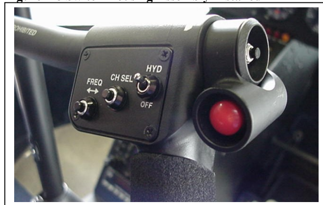
Figure 2-8 Switch Housing Assembly Installed
