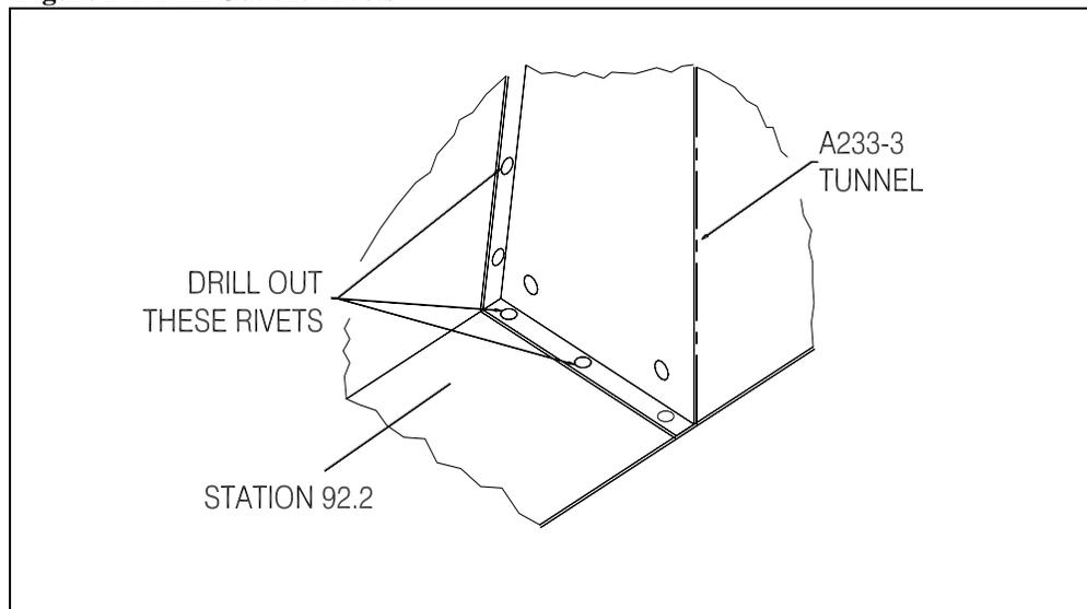
6. Position the Mount Block tight in the corner against the aft side of the firewall (A233-1) and the left side of the tunnel (A233-3). Ensure that the upper hole in the Mount Block is aligned with the existing hole\* in the tunnel. Drill out the existing upper hole in the tunnel to 0.189 with a #12 drill (reference Figure 2-3).
