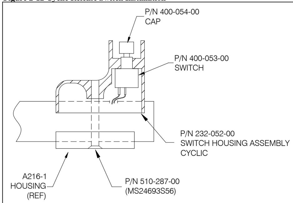
8. Install the P/N 400-053-00 switch in the P/N 232-052-00 cyclic switch housing assembly using needle nose pliers to hold the switch. Install the completed switch housing assembly with the correct hardware as shown in Figure 2-12, by removing the existing A216-1 housing screw and replacing it with the longer P/N 510-287-00 screw. Re-install the A216-1 housing and wires.
