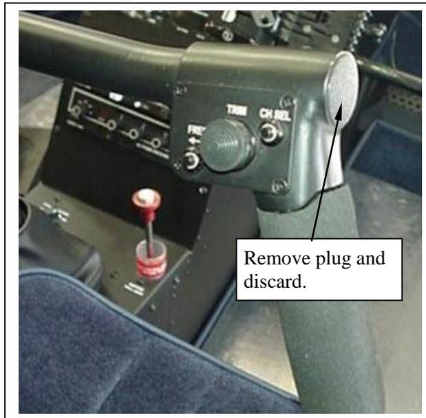
2. Remove outboard screw (MS27039C0806) and nut (MS21042L08) as shown in Figure 2-14.
