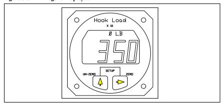
The illustration is a typical hook load reading. The display is 3,500 pounds, note the last digit is not displayed.
