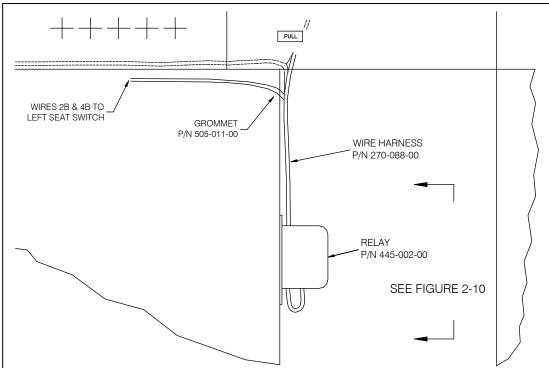
Figure 2-9 Wire Harness and Relay Installation
