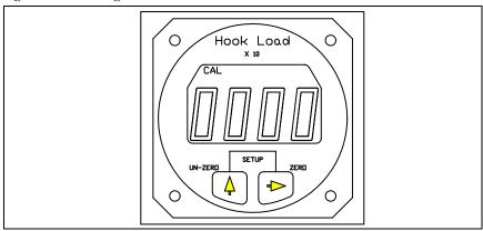
The CAL legend is turned on and the first digit is blinking. The previous load is not displayed. At this point if you wish to return to the Run Mode without changing the Calibration Code, power cycle the Indicator. At this point it is not possible to return to the Run Mode without changing the Calibration Code by using the buttons on the Indicator front panel.
