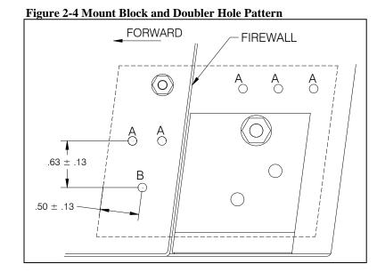
13. Drill the remaining two holes in the Mount Block and tunnel through the doubler with a .189 inch #12 drill bit.
