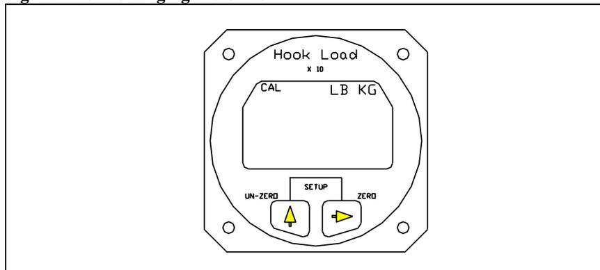
The CAL legend is turned on and the previously set unit is displayed. To return to Run without changing the units, press both the Right and Left Button at the same time. To change the units press the left button. When the selection has been made, press both the Right and Left Button at the same time to return to Run.
