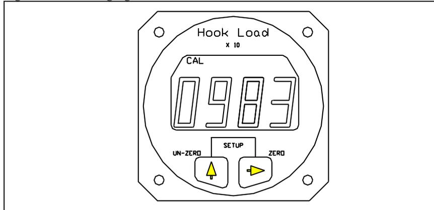
The CAL legend is turned on and the previously entered or computed Calibration Code is displayed. To return to Run without changing the CAL Code, press both the Right and Left Buttons at the same time. To change the Calibration Code, use the right button to select the digit to be changed, then use the left button to scroll the blinking digit to the desired number. When the Calibration Code has been entered, press both the Right and Left Button at the same time to return to Run.
