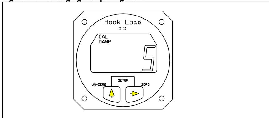
The CAL and the DAMP legend is turned on and the previously set dampening level is displayed. To return to Run without changing the current dampening level press both the Right and Left buttons at the same time. To change the dampening number, use the left button to scroll the blinking digit to the desired number. After the selection has been made press both the Right and Left buttons at the same time to return to Run.
