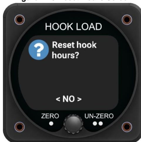
Figure 4.15 Reset Hours Screen
