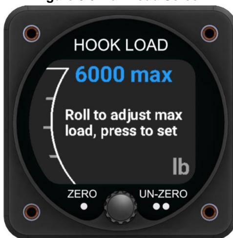
Figure 3.5 Max Load Screen
