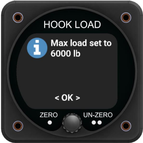
Figure 4.5 Max Load Confirmation Screen
