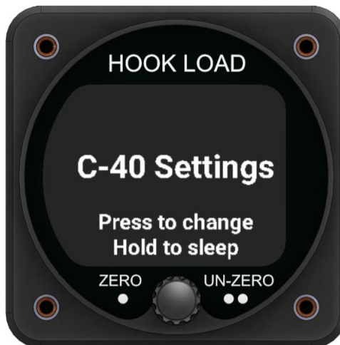
Figure 3.7 Turning the Display Off
