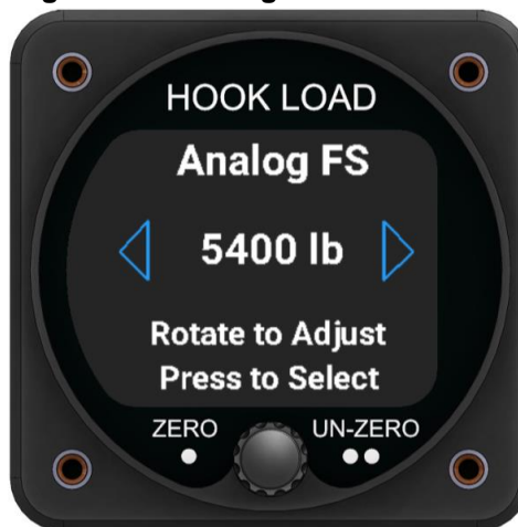
Figure 4.14 Analog Full Scale Screen
