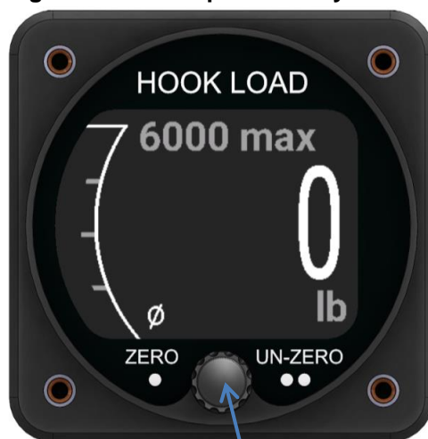
Figure 3.3 User Input – Rotary Knob
