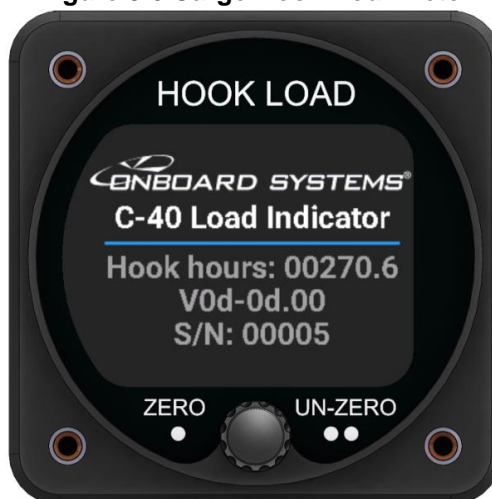
Figure 3.6 Cargo Hook Hour Meter
