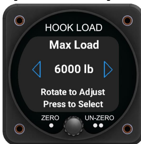
Figure 4.4 Max Load Setting Screen
