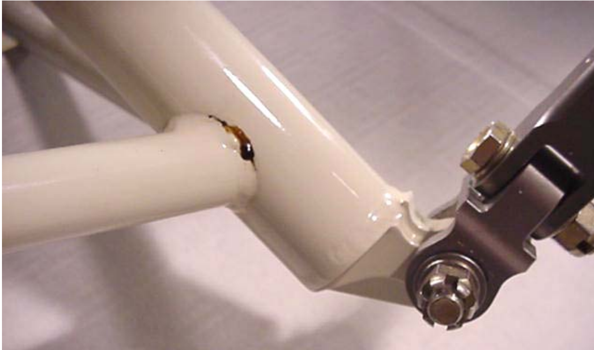
Typical crack with corrosion preventative oil leaking out.
