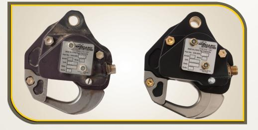
When you send your cargo hook to Onboard Systems for overhaul, we restore it to likenew condition. Here are unedited photos of a TALON LC Keeperless hook (P/N 528-029-00) before overhaul (on the left), and after overhaul (on the right). +
