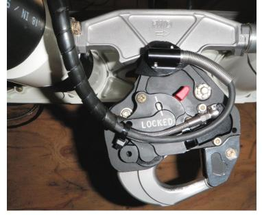
Figure 2.3.3 Pin Load Cell Harness Routing (P/N 210-226-02 shown)
